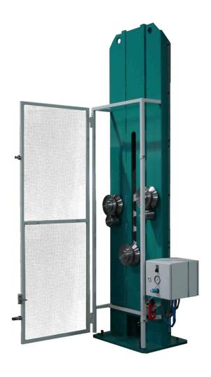
Turn-Off device on basis of a 3-roll system Middle roll is movable in case of a pay-off interruption (overcharge) Provides an "Emergency-stop" signal to the drawing machine control
