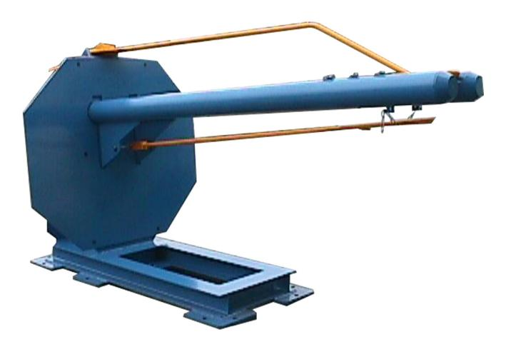
Flipper with a coil weight capacity up to 2 t Sturdy double pipe steel construction Including wire "hold-down" device Side by side lineup for continiously wire payoff Loop accumulator as wire break protection (optional)
