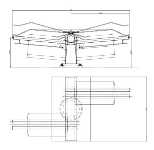
Double Flipper with a coil weight capacity up to 2 x 2 t Two payoff cones displaced on 180° Manual rotatable Including wire "hold-down" device Sturdy double pipe steel construction Loop accumulator as wire break protection (optional)
