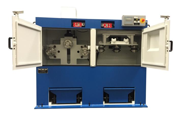
2 x 3 bending rolls with long lifetime tungsten carbide inserts
