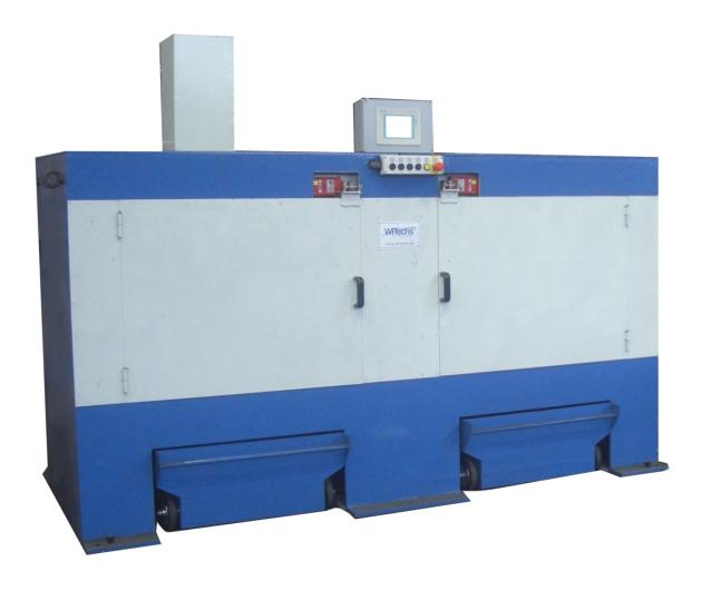
2 x 3 extra sturdy bending rolls with long lifetime tungsten carbide inserts Bending and breaking of scale in 2 levels (4 directions)
