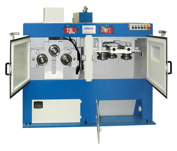
2 x 3 bending rolls with long lifetime tungsten carbide inserts
