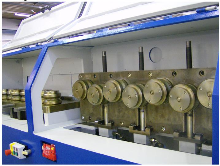
2 x 7 bending rolls with long lifetime tungsten carbide inserts
