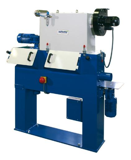
For coating wire with lubricant soap Mainly used for concrete reinforcement steel wire coating before cold rolling Perfect homogeneous coating (reproducible) Coating and dust collecting bay with screw conveyor Including integrated extraction system
