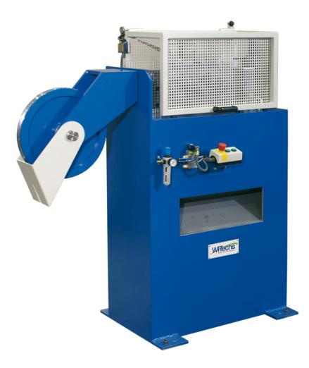
Improves the tensile strength to yield strenght (Rm/Re) ratio Improves the total uniform elongation (Agt) Stress relieving of the wire rod due to a proven 5 roller straightening unit Presetting of the upper stress relieving rollers pneumatically (hydraulically as an option) cylinder Adjustable via threaded spindle
