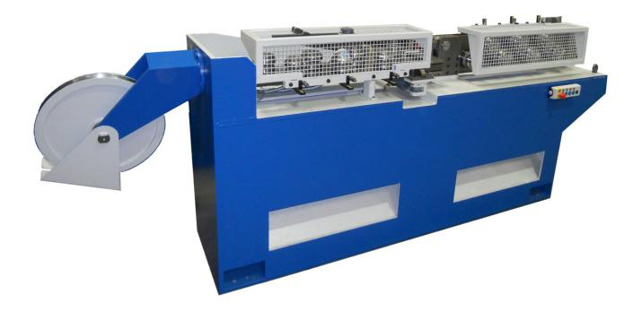
Improves the tensile strength to yield strenght (Rm/Re) ratio Improves the total uniform elongation (Agt) Stress relieving of the wire rod due to a proven 7 roller straightening unit Presetting of the upper stress relieving rollers pneumatically (hydraulically as an option) cylinder Adjustable via threaded spindle
