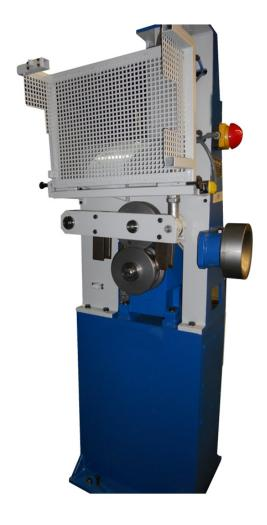
Pull-in device to pre-feed wire rod within a drawing line Setting of one feeding roller by means of a pneumatic cylinder Electrically driven feeding roller
