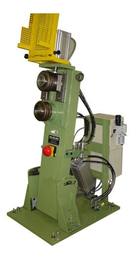
Pull-in device to pre-feed wire rod within a drawing line Setting of one feeding roller by means of a pneumatic cylinder Hydraulically driven feeding roller Swivel mounted design, during production the unit can be tilted out of the wire rod area
