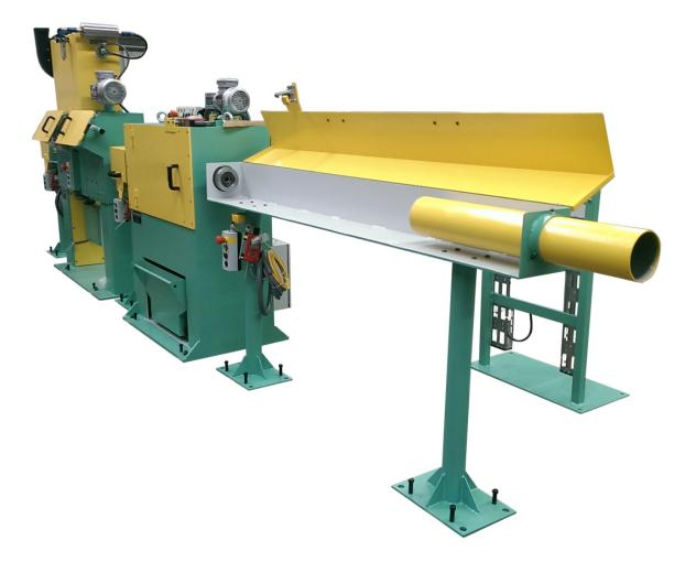
To protect staff against accidential contact to the passing wire rod Adjustment of protection area at place possible
