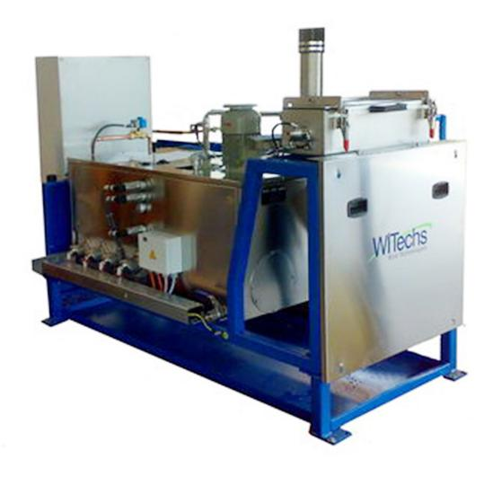
High pressure wire cleaning (rinsing) with hot water before drawing Including high efficient cold and hot air drying system
