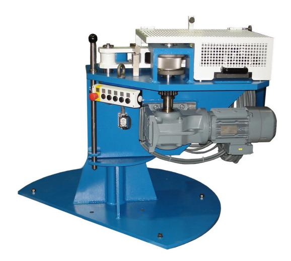
Pull-in and straightening device to pre-feed wire rod within a drawing line Setting of one feeding roller by means of a hydraulic cylinder Electrically driven feeding roller Including 5 Roller straightening device Swivel mounted design, during production the unit can be rotated out of the wire rod area Hydraulic aggregate in scope of delivery
