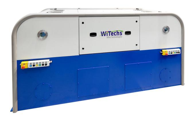
For cleaning sanding or removing surface defects by means of 2 sanding belts as well as optionally by means of a pressing device
