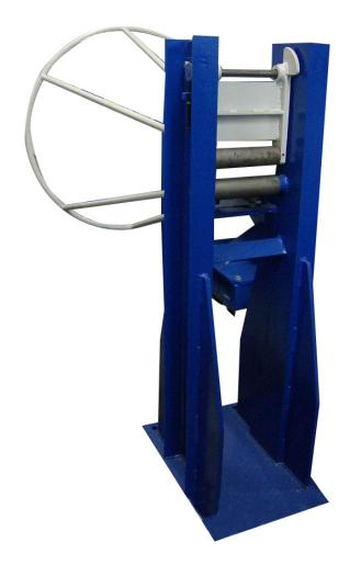
Suitable to detect wire rod tangles, knots etc. Provides an "Emergency-stop" signal to the drawing machine control Wire guiding and levelling due to a wire rod inlet basket
