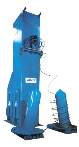
Tower height approx. 8 - 9 m Hydraulically tiltable pay-off cones, coil weight capacity up to 3 t Closed, heavy duty construction Upper guiding roller movable by means of a chain host
